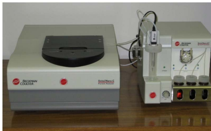
Delsa™ Nano Zeta Potential and Submicron Particle Size Analyzer, Beckman Coulter Inc.
